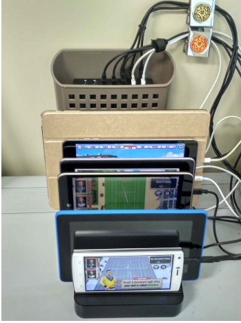
Figure 3: A prototype mobile farm with eight connected devices.
